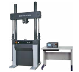
Inspecting Hydrogen-Related Part Strength Fatigue and Endurance Testing Machine
