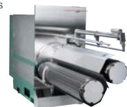
Manufacturing Glass Fibers for Reinforcing Turbine Blades Glass Winder
