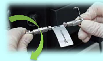
(Previous) Manual connection of packed columns
