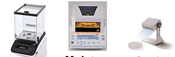
Balance Moisture Analyzer Static Eliminator
