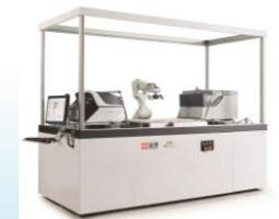
Automated EDX system with 540 samples per cycle
