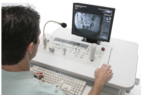
Fig. 9 I.I.-DR Model with 1-Megapixel CCD
