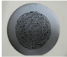
Fig. 3 Test Specimen Showing Random Pattern
