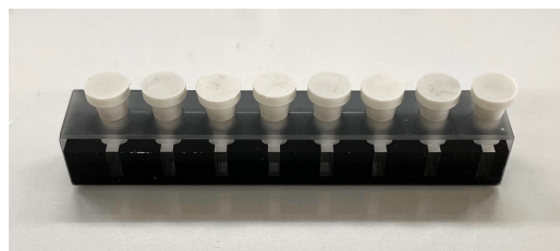
Fig. 3 Dedicated 8-Series Micro Cell (Pathlength: 10 mm)
