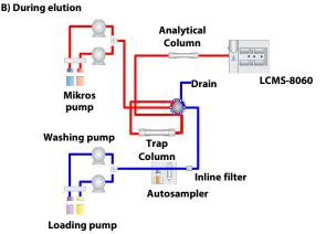
Fig. 2 Flow Diagrams of Trap and Elute System
