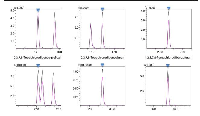
Fig. 1 Chromatograms of Representative Compounds in Analysis of Standard Samples (Concentration: 0.025 pg/µL)
