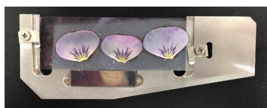
Fig. 3 Samples Mounted in Dedicated Holder (ITO Slide Glass)
