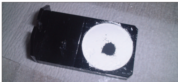
Fig. 1 Sample Placed on \text{BaSO}_4 Powder
