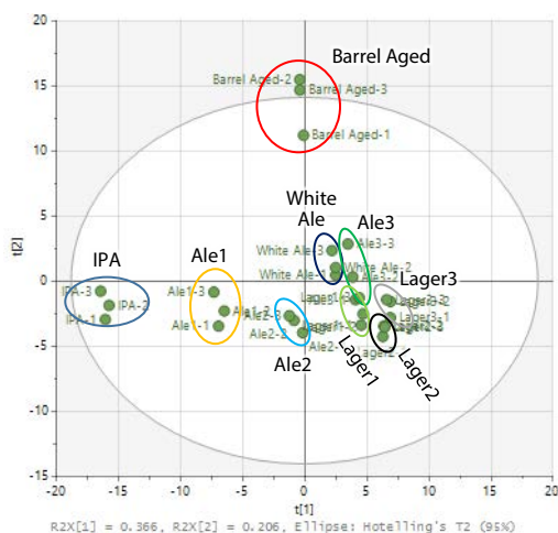
Fig. 2 PCA Score Plot for Data from the Analysis of Aromatic Components in 9 Commercially Available Beers
