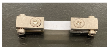
Fig. 3 View of the Sample and Chucks
