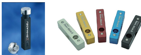
Fig. 2 Left: TrayCell Right: Nano Stick
