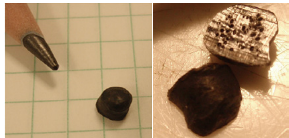
Fig. 28 (Left) Approx. 5-mm Diameter Plastic Pellet (Right) Cross Section
