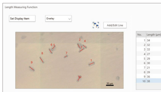
Fig. 15 Length Measurement Operation Screen and Measurement Length Results
