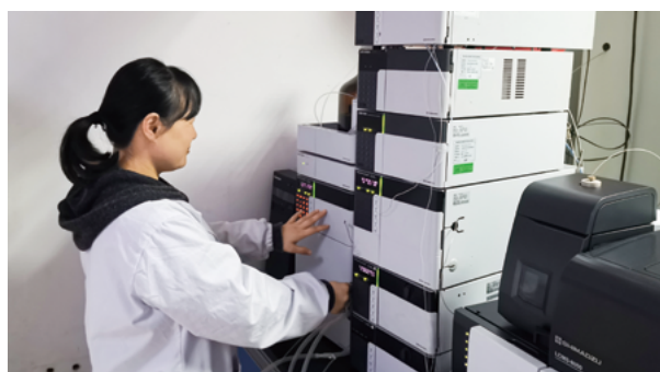
Photo: Customer of Institute for Food and Drugs Control use LCMS-8050 to detect NDMA in metformin
