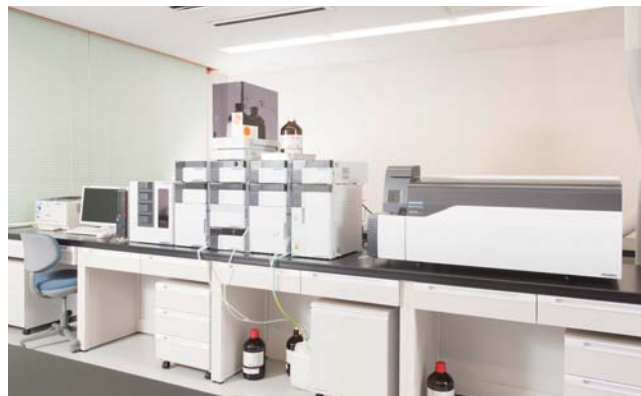
The first unit of the Nexera UC supercritical fluid extraction/chromatography system
