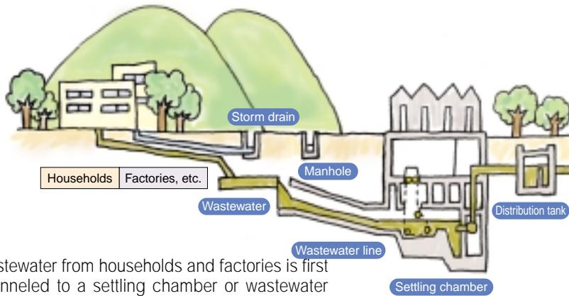
Wastewater from households and factories is first channeled to a settling chamber or wastewater pump room, where large pieces of garbage and soil are removed.
