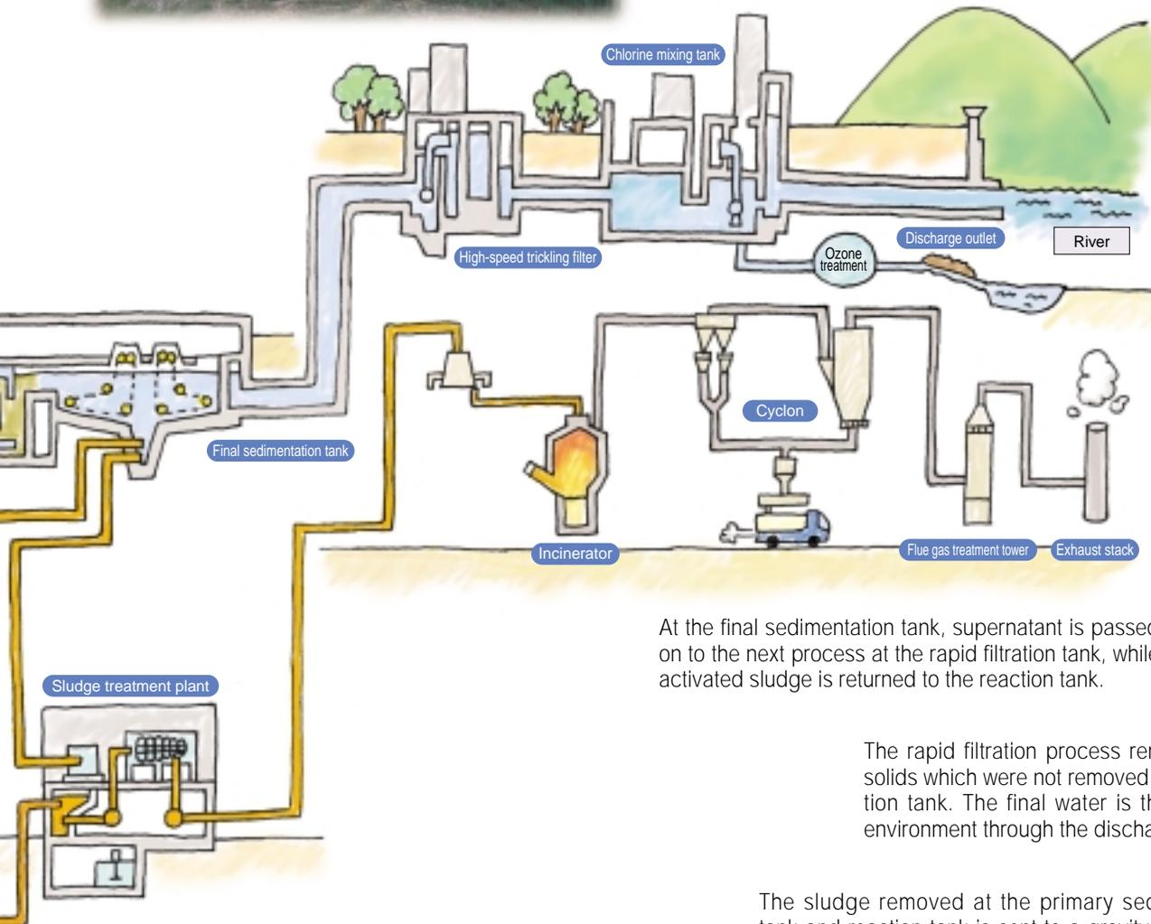
At the final sedimentation tank, supernatant is passed on to the next process at the rapid filtration tank, while activated sludge is returned to the reaction tank.
