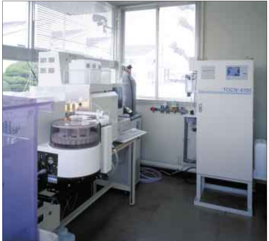
Continuous wastewater monitoring system at Shimadzu main works TOC and TN by Total Organic Carbon/Total Nitrogen Continuous Monitor, TOCN-4100 Heavy metals (Ni, Cu) by Atomic Absorption Spectrophotometer, AA-6650
