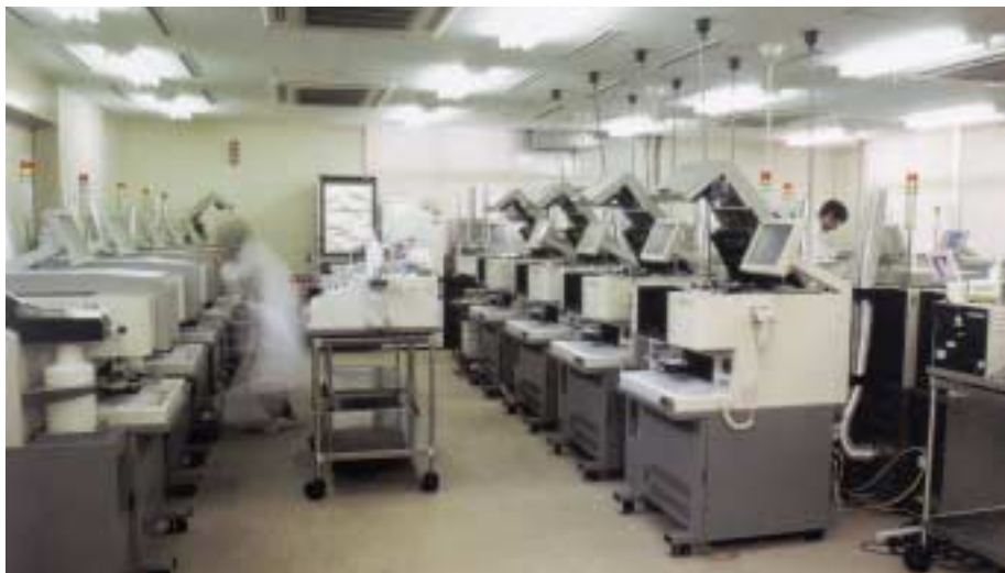
Large-scale gene analysis using Shimadzu's world-fastest DNA sequencers, RISA-384 at the Institute of Physical and Chemical Research.
