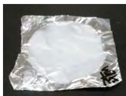
Fig. 3 Wood-Derived CNF Applied to and Dried on Aluminum Foil
