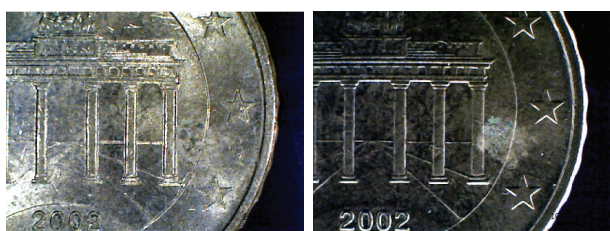
Fig. 2 Observation Images of Coin Surface Captured Using the Wide-Field Camera Left: Bright State, Right: Dark State
