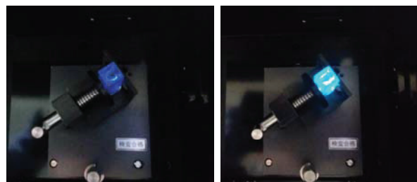
Fig. 2 Cell Set on the Solid Sample Holder Left: Low Concentration ( 1.0 \times 10^{-4} mol/L), Right: High Concentration ( 1.0 \times 10^{-2} mol/L)
