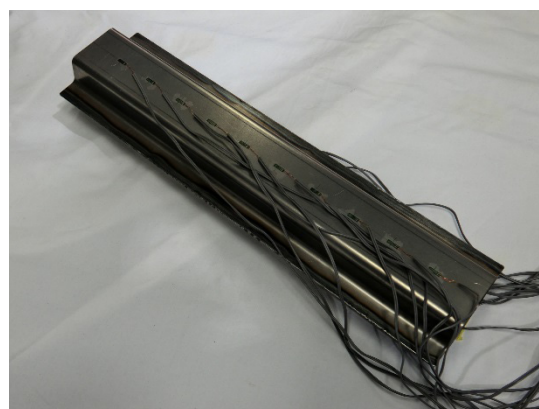
Fig. 2 Test Specimen after Attaching Strain Gauges (High Tensile Strength Steel)
