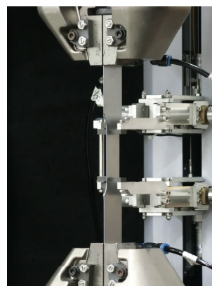
Fig. 3 Specimen and Jigs for Tensile Testing
