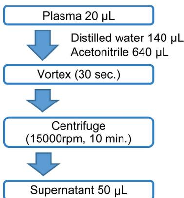
Fig. 1 Pretreatment Workflow of Blood Plasma Samples
