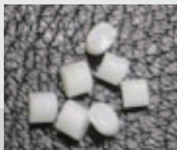
Thermal Extraction of PS Plastic Shavings (1 mg) for 5 Minutes at 300°C
