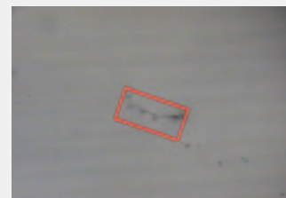
Microscope Photograph of Foreign Substance on Film Red box: 50 \times 100 \mu\text{m}
