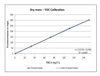
First, the algae sample is measured and the TOC is determined. Subsequently, the sample is filtered through a 0.2  $\mu$ m syringe filter and measured again in the TOC analyzer to be able to distinguish between the TOC content originating from the algae and the carbon content possibly originating from
