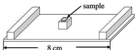
Fig. 1 Handmade tool for polishing.
