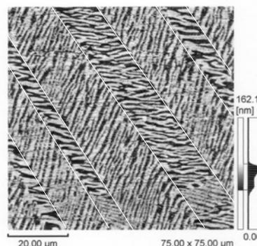
Fig. 2 Topographic image on ferroelectrics by AFM.
