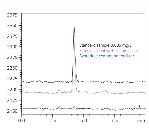
Fig. 4 SIM Chromatograms of STD and Fertilizer Sample
