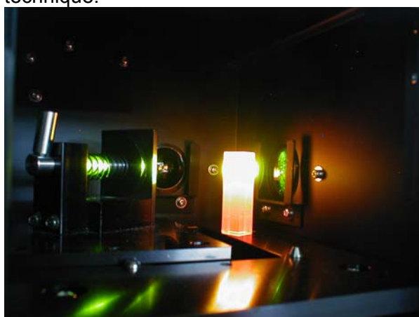
Fig. 1: View into the sample compartment of the Shimadzu RF-5301PC, inclusive solid sample holder and a Rhodamine B bloc, which was brought to excitation.
