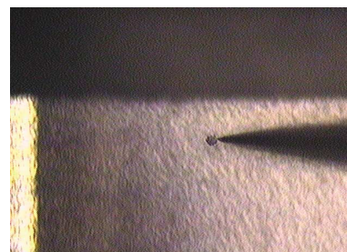
Fig.3 Picking out Micro Contaminant using Metal Probe
