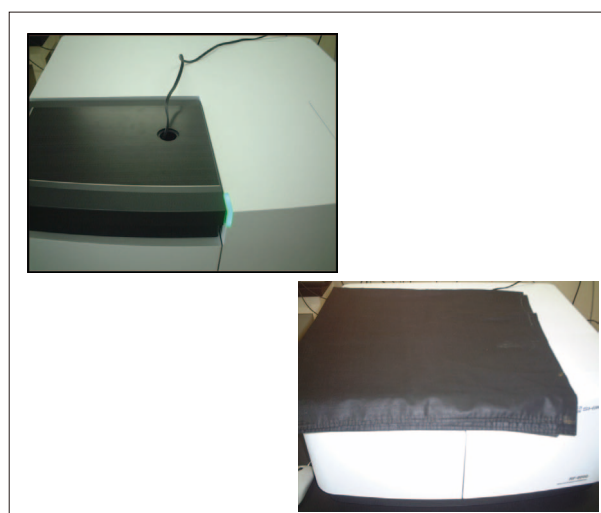
Fig. 3 Measurements with Sample Compartment Covered with Blackout Cloth
