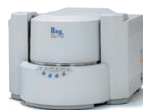
Fig. 5 Photograph of EDX-800HS Energy Dispersive X-Ray Fluorescence Spectrometer
