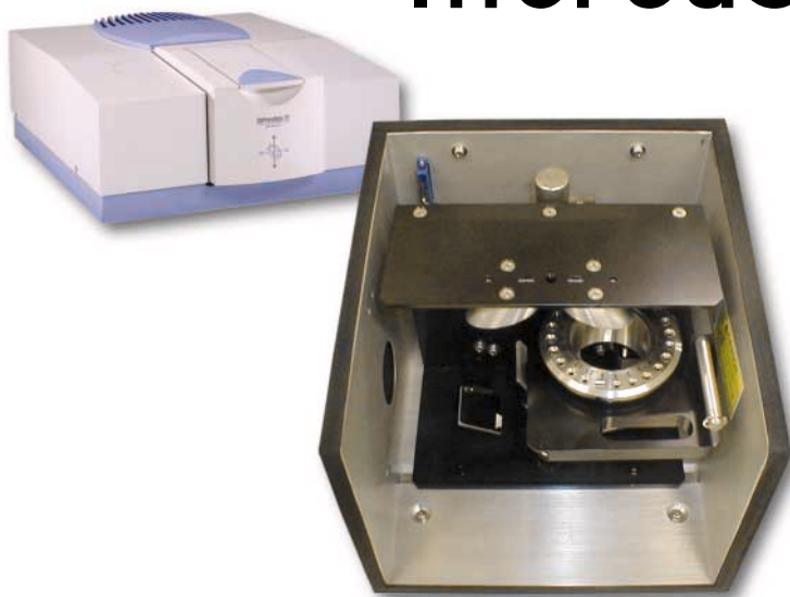
Figure 1: DRS-8010ASC for 24 samples with the diffuse reflection unit based on elliptical mirrors in the 'praying mantis' configuration
