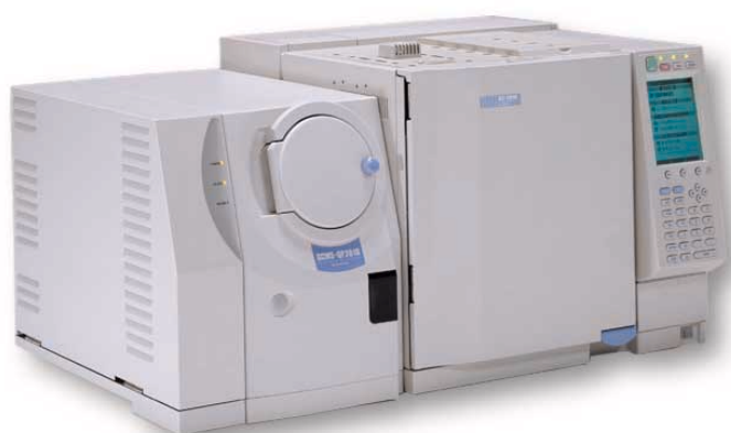
The highly sensitive quadrupole mass spectrometer GCMS-QP2010
