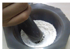
Fig. 2 Homogenization by Pulverizing
