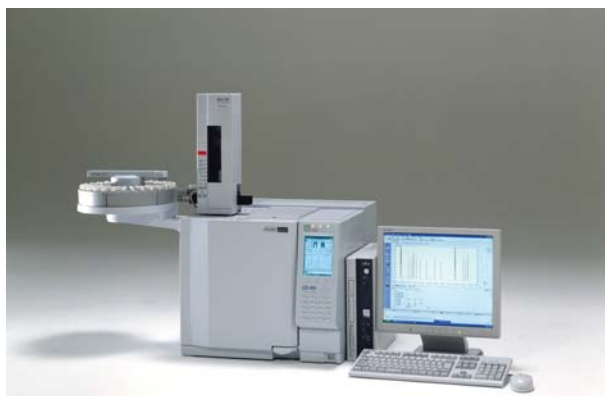
GC-2010AF Gas Chromatography for BioDiesel Analysis.
