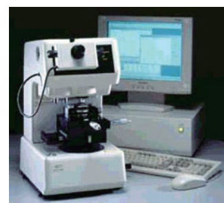
Fig. 1 Overview of Shimadzu MCT-W500 Micro Compression Testing Machine
