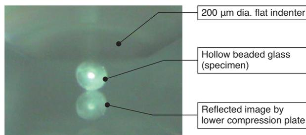
Fig. 4 Example of Observed Image of Specimen
