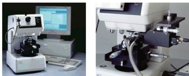
Fig. 1 Overview of MCT-W500 Micro Compression Testing Machine (with Side Observation Kit)
