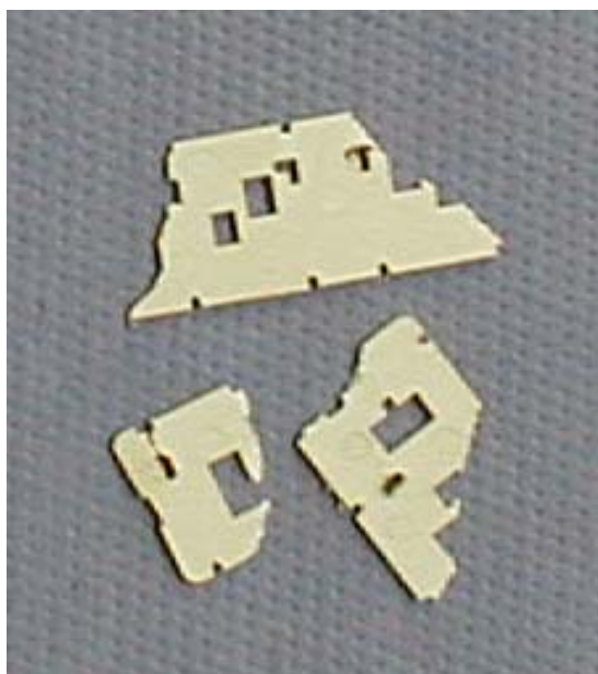
Fig. 1: Polymer elements to be analyzed, regards the presence of brominated flame retardants
