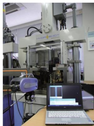
Fig. 2 Setup of High-Rate Tensile Test and Video Recording
