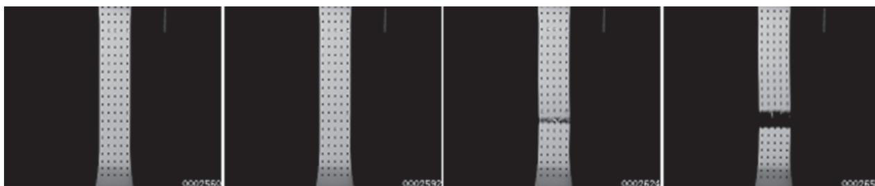
Fig. 3 Four Frames of Specimen Before and After Breakpoint
