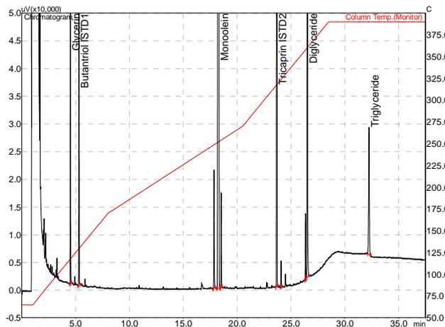
Fig. 2: Chromatogram of a Biodiesel standard
