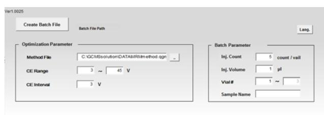
To use the MRM optimization tool, just set the parameters shown in the figure on the left to automatically create multiple method files (product ion scan mode) and batch files with the CEs configured. Using the batch file, start a consecutive product ion scan analysis.
