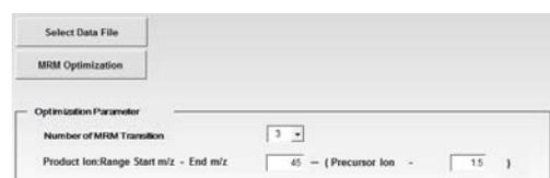
Transitions can be optimized to select the data files obtained through measurements using the MRM optimization tool. Fig. 1 shows the graph of transitions and CEs. CEs were optimized with high accuracy.
