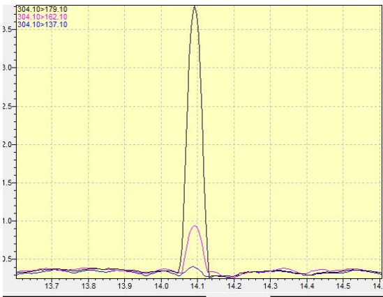
Figure 4B: MRM Chromatograms Diazinon at 5 ppb in Orange Oil
