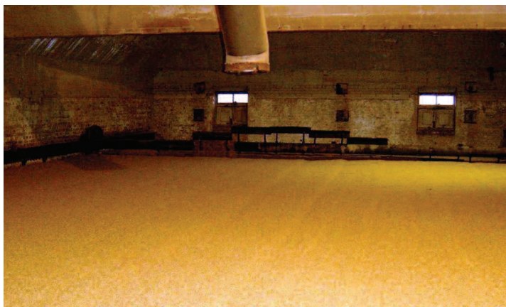
Figure 2: Traditional direct fired floor kiln (capacity ~ 20 t)
