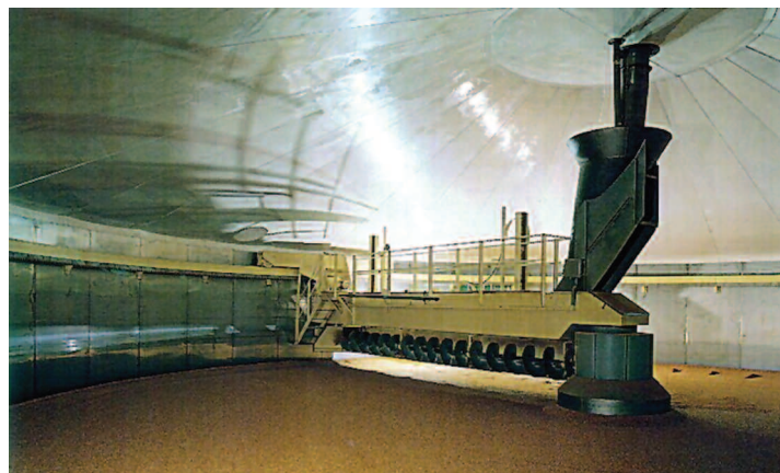
Figure 3: Modern indirect fired kiln (capacity ~ 200 t)
