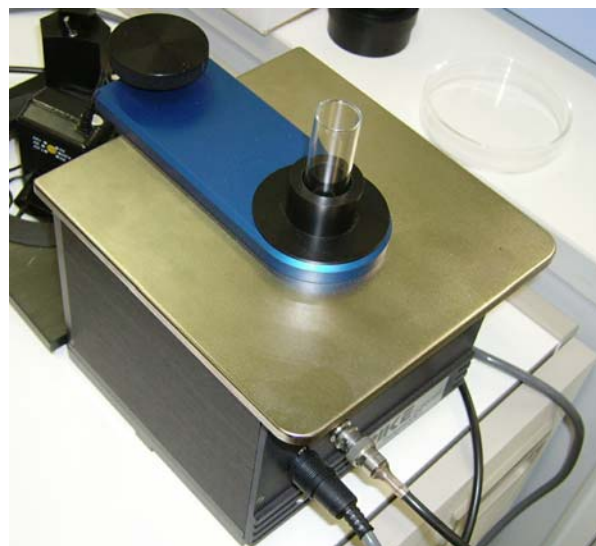
Fig. 4: IntegratIR, an accessory with built in InGaAs detector, designed as integrating sphere for the FT-NIR measurement for solid material like powders, etc.
