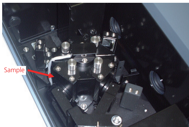
Fig. 2 Sample Set in Integrating Sphere
