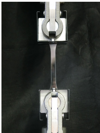
Fig. 1 Tensile Test of the Resin Specimen
