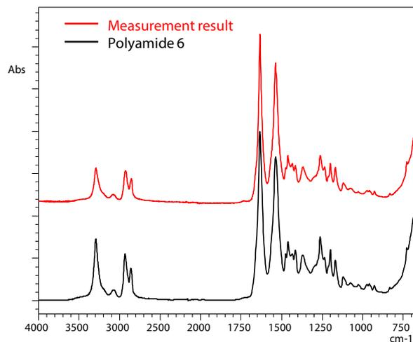
Fig. 5 IR Spectrum of Thermoplastic CFRP Using Polyamide 6
