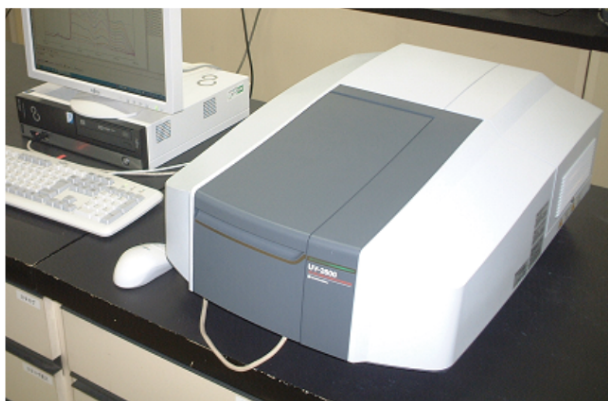
Fig. 2 UV-2600 with Mounted Integrating Sphere Attachment
